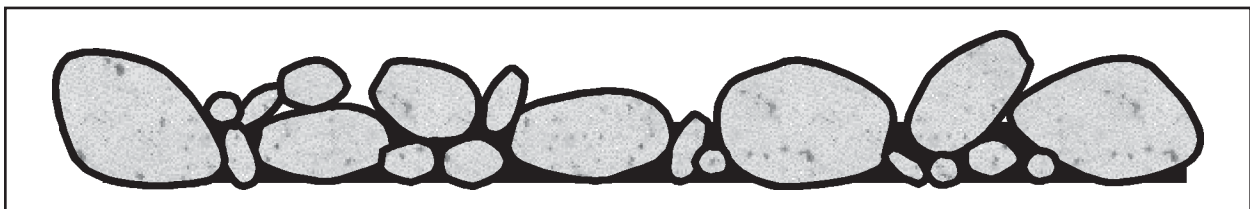
Figure 3.2.5. Cross section of a graded chip seal aggregate
