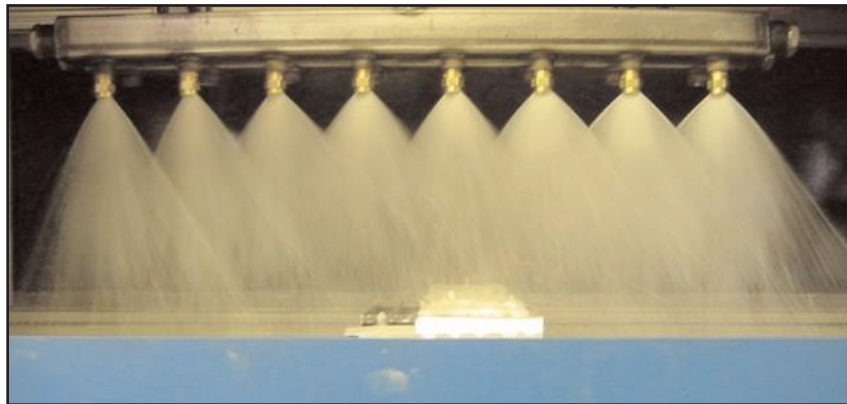
Figure 3.8.8. Spray bar nozzle showing proper alignment
