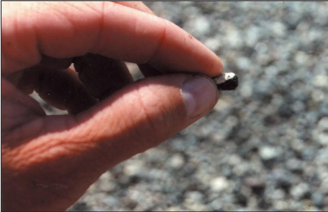
Figure 3.4.3. Proper embedment (~70%) into the residual asphalt
