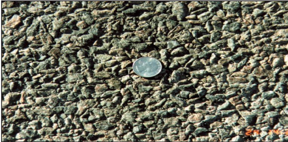
Figure 3.2.6. Example of a one-size FA-4 chip seal aggregate
