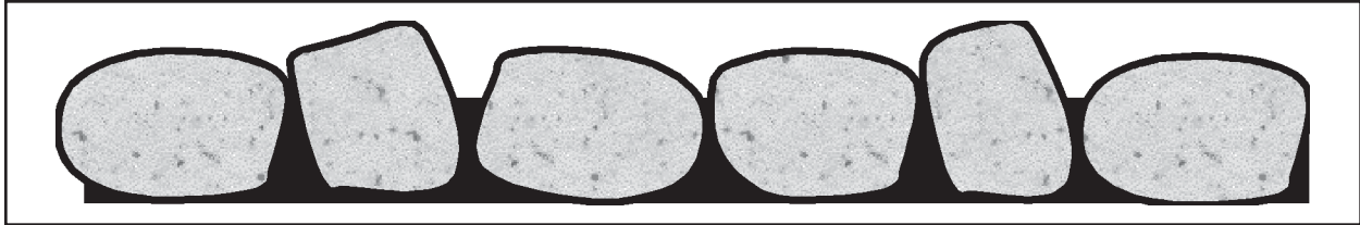
Figure 3.2.4. Cross section of a one-size chip seal aggregate
