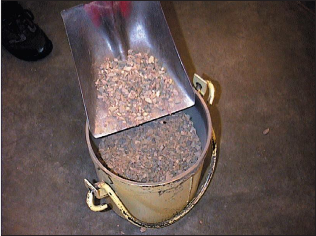
Figure 3.4.6. Loose Unit Weight Test
