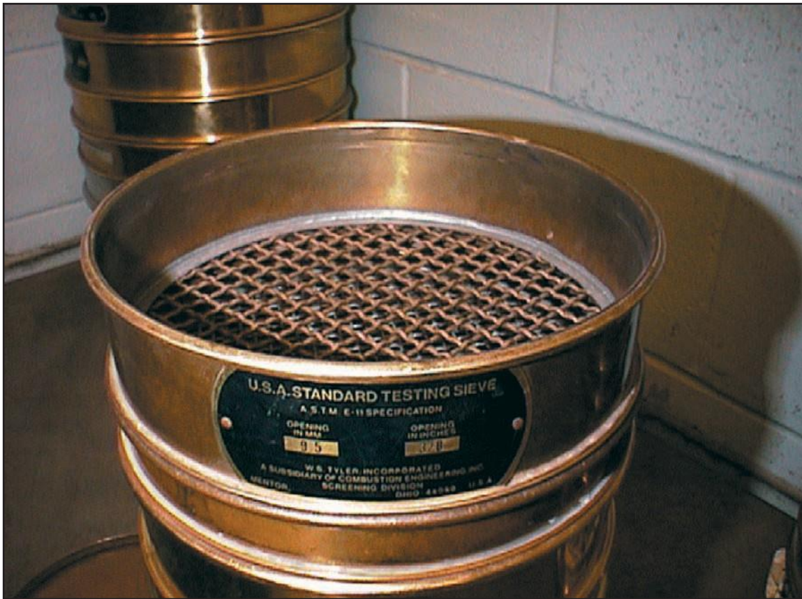
Figure 3.4.4. Chip seal Sieve Nest
