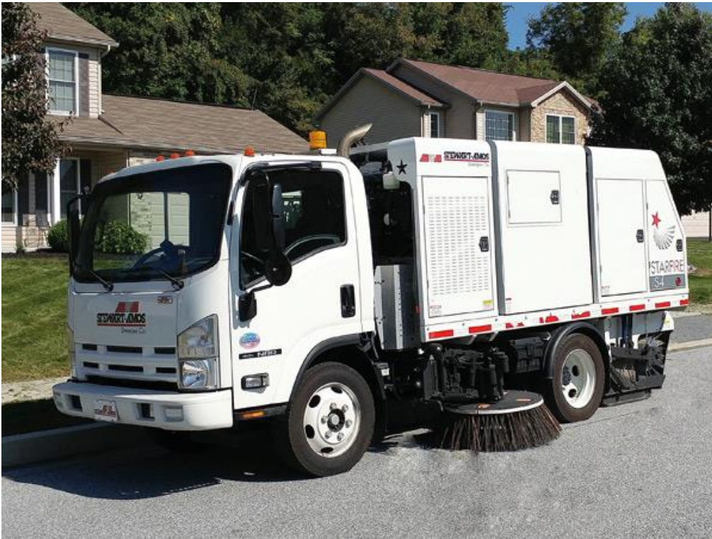
Figure 3.1.4. Pick-up sweeper typically used in urban areas
