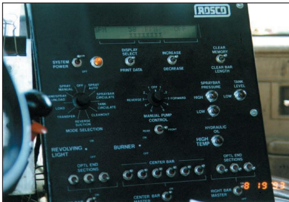
Figure 3.1.6. Computer control console of an asphalt distributor
