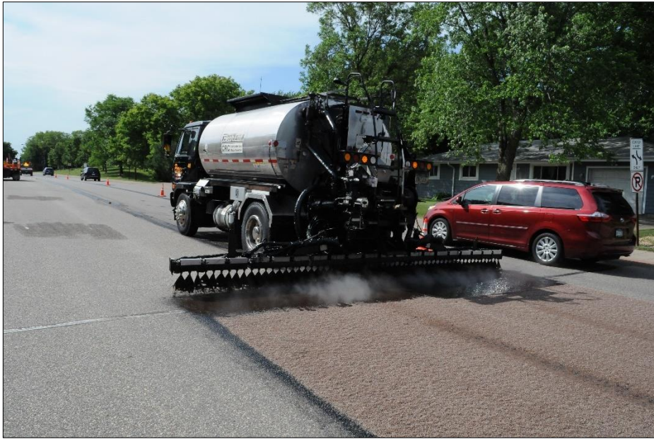
Figure 3.1.5. Computer controlled asphalt distributor
