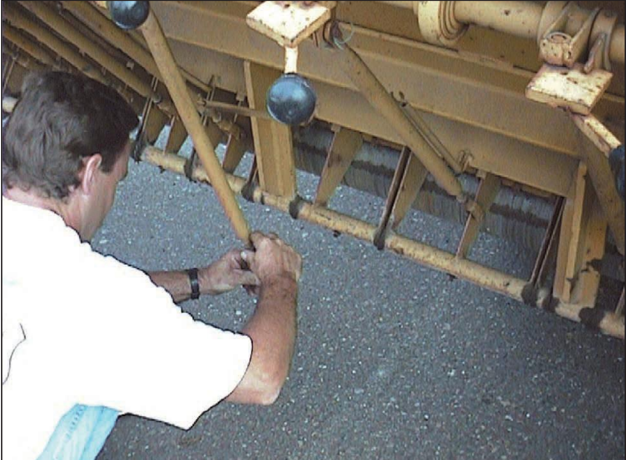
Figure 3.8.5. A spreader gate is adjusted
